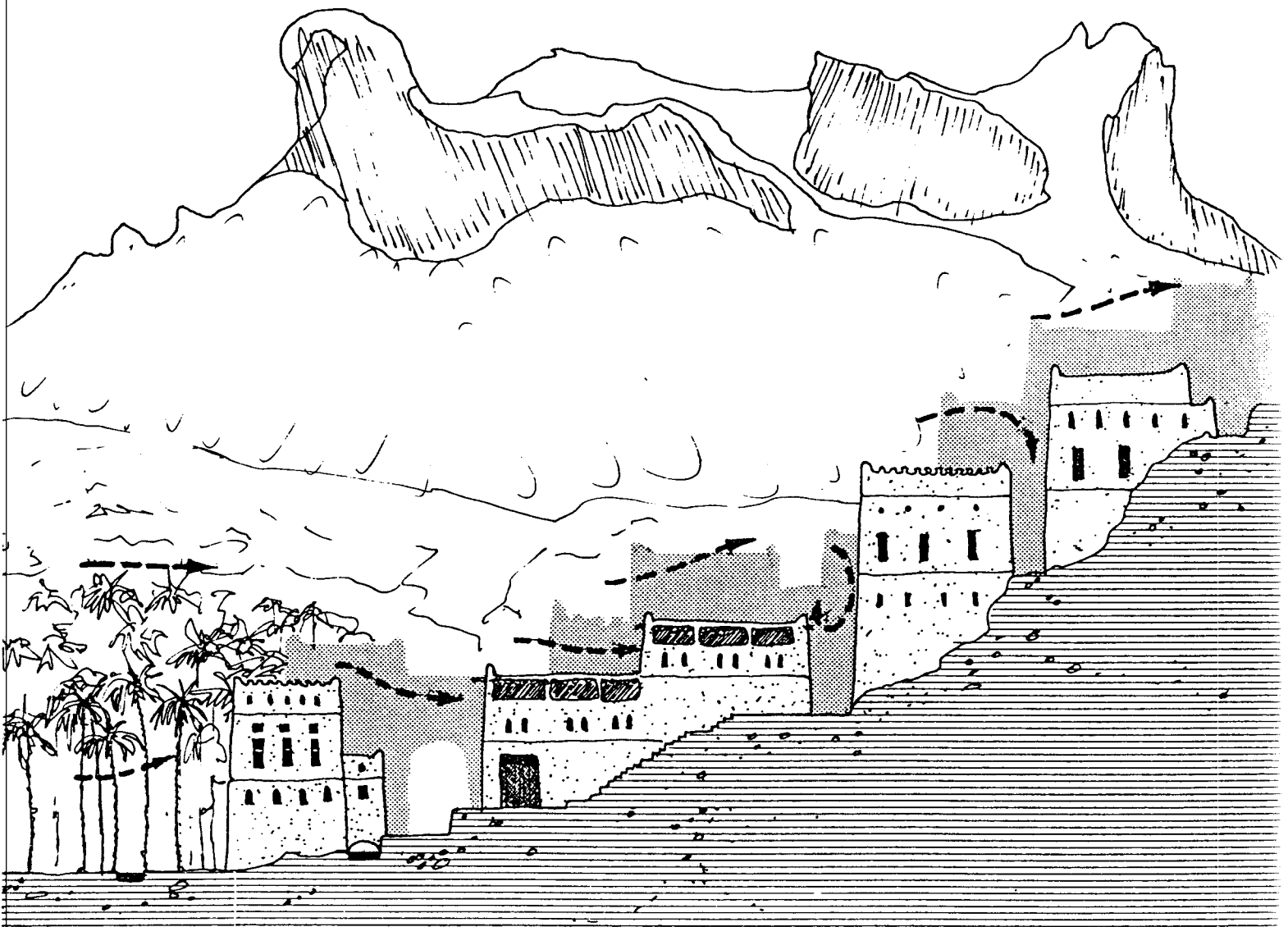
Fig 406. Schematic section through Al Hamrah showing the effect of up-slope valley winds.
