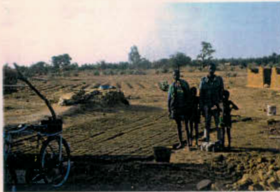
Above: at the end of the day, small roofbricks are left to dry. (Sevare, Apr '95)
